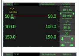
If dual frequency transducers are installed then the frequency button will allow the user to change between the available frequencies.
