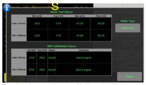
The values shown should be below 20mV once installed unless otherwise stated. High values can usually be reduced by improved cabling and / or filters on the power supply.
