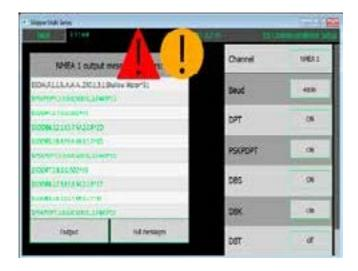
If connected to a central alarm management system, and this fails, the lack of an HBT NMEA message from the CAM will cause the system to take back control after a little more than a minute.
