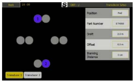
If only one transducer is installed (to transducer 1) then "Transducer 2" must be set to position "Not connected".
