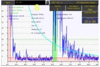
Here you can see the pings and the parameters in use to detect it, The green zone is showing the detected depth, the red zones are areas where the bottom detection will not have an effect. This is typically at low signal levels and in the ringing period after the system sends a pulse.
