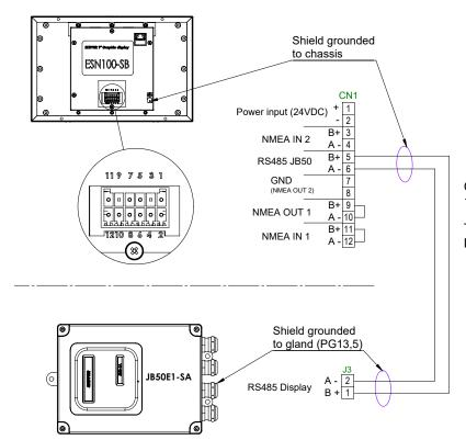
Cable: RS485, baud rate 115200 1-pair twisted and shielded
