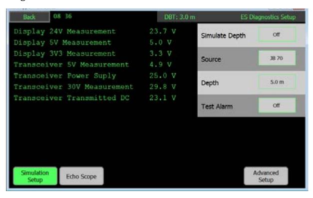
The ESN100 has a number of functions to allow the user to simulate, diagnose and optimise the system.
