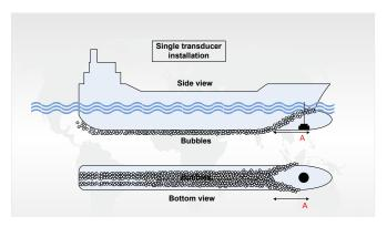
The transmitting surface of the transducer must be installed horizontally with no more than 5 degrees tilt. If this is not possible a blister should be assembled. This should have at least 0.3m of flat area around the transducer, and be tear drop shaped.
