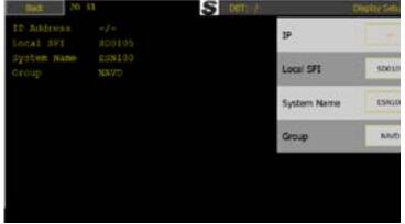
This standard requires a unique identifier for this equipment this is called the System Function Identifier (SFI). This is set by default to SD0105, but can and should be changed if more than one device on the network. The SFI is made up of 2 letters 'SD' as designated for an echosounder, and 4 digits from 0001 to 9999. This is used to allow the equipment to identify itself to other equipment, and to filter which messages are aimed for this device.
