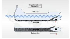
Larger vessels are often fitted with two transducers, one fore and one aft (see fig.) The fore transducer is the primary transducer, (normally 50 kHz).
