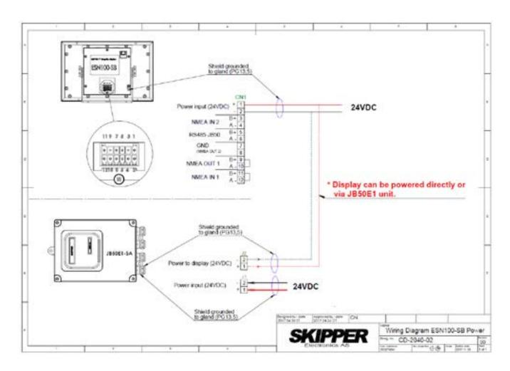
Power input circuitry inside JB50E1-SA with resettable fuse 2,5A (at 20deg C) power on/off switch and available 24VDC output to display unit.
